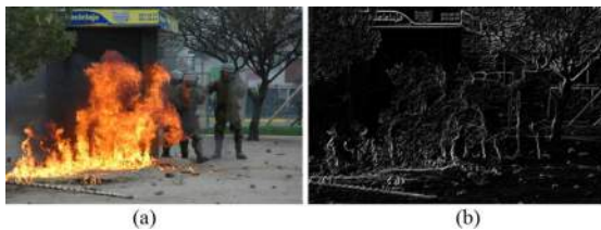
Figure 6: (a) Original Image (b) Gabor filter with a kernel setting.
